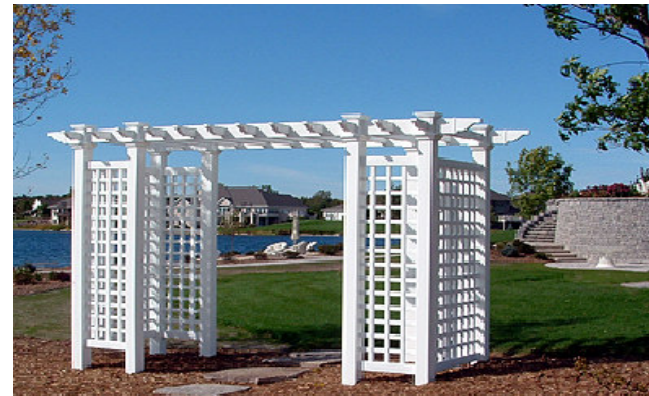
Approximately 5' x 16' pergola Free standing 1 1/2" x 5 1/2" beams 2" x 3 1/2" joists Built in lattice
